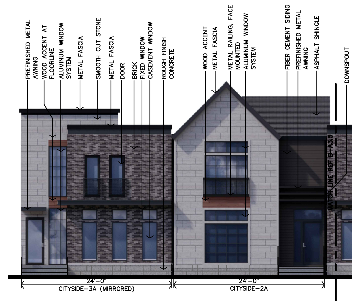
D BUILDING 5 STREET ELEVATION 1/8"=1'-0"
