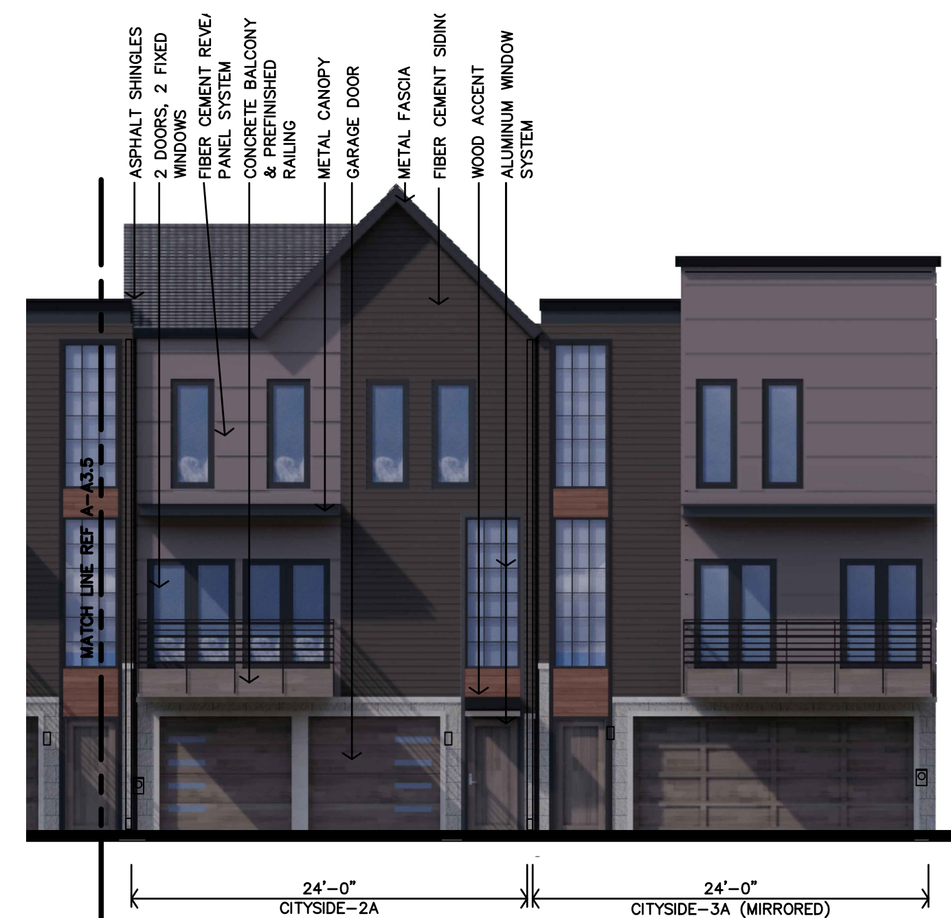
B BUILDING 5 GARAGE ELEVATION 1/8"=1'-0"
