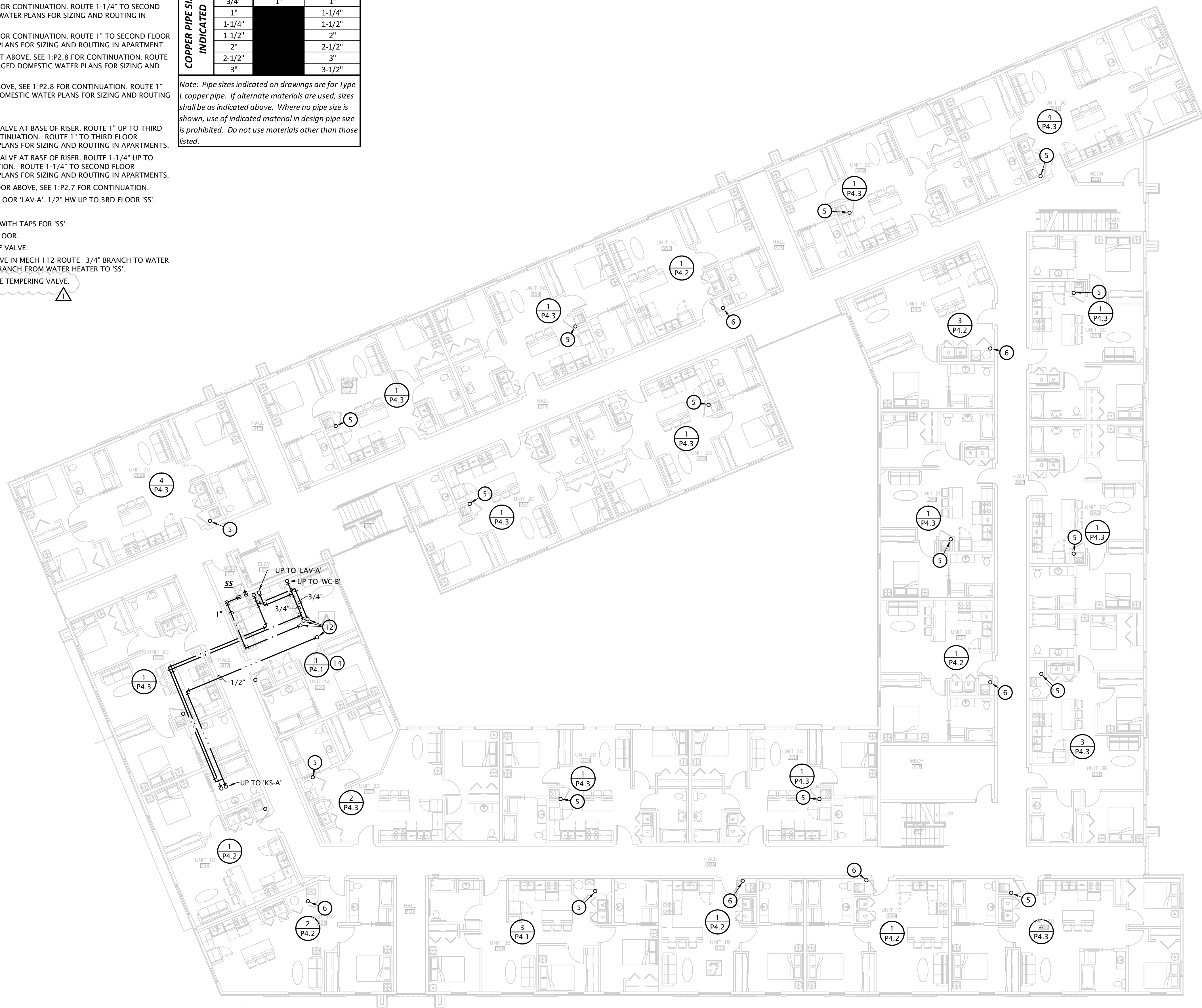
1 THIRD FLOOR PLAN - DOMESTIC WATER 3/32" = 1'-0"
