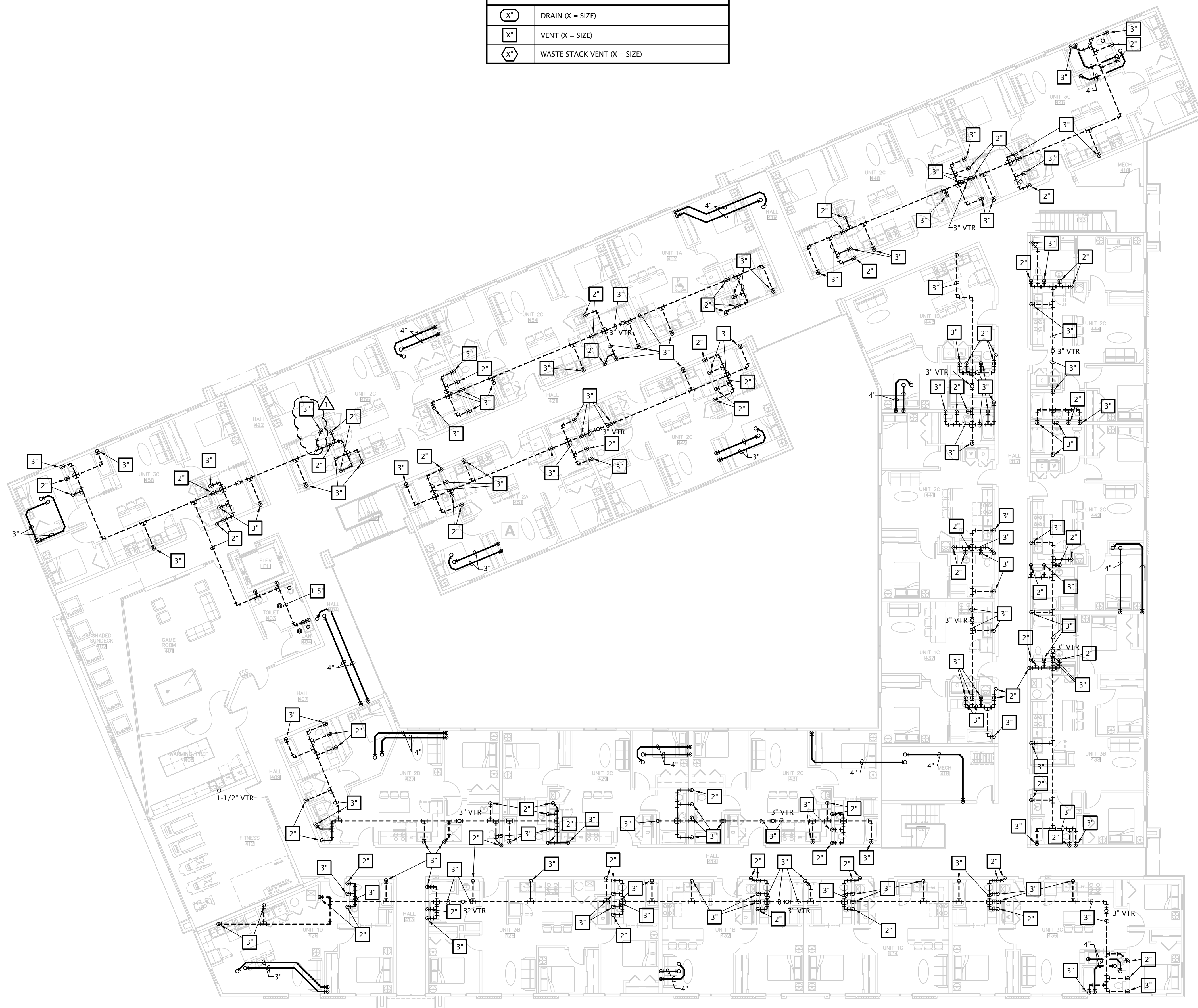
1 FOURTH FLOOR PLAN - DRAIN AND VENT 3/32" = 1'-0"
