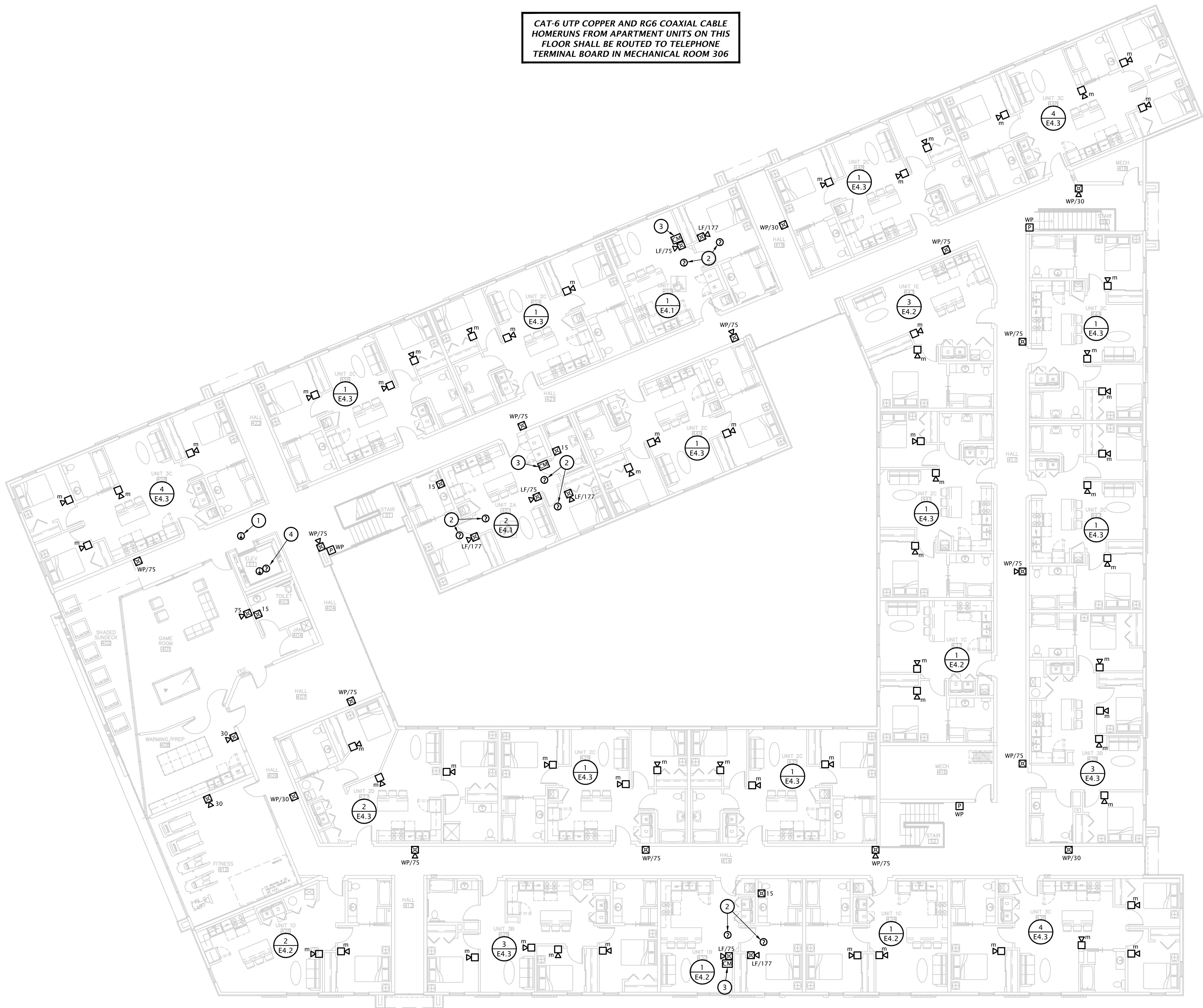
① FOURTH FLOOR PLAN - SPECIAL SYSTEMS 3/32" = 1'-0"
