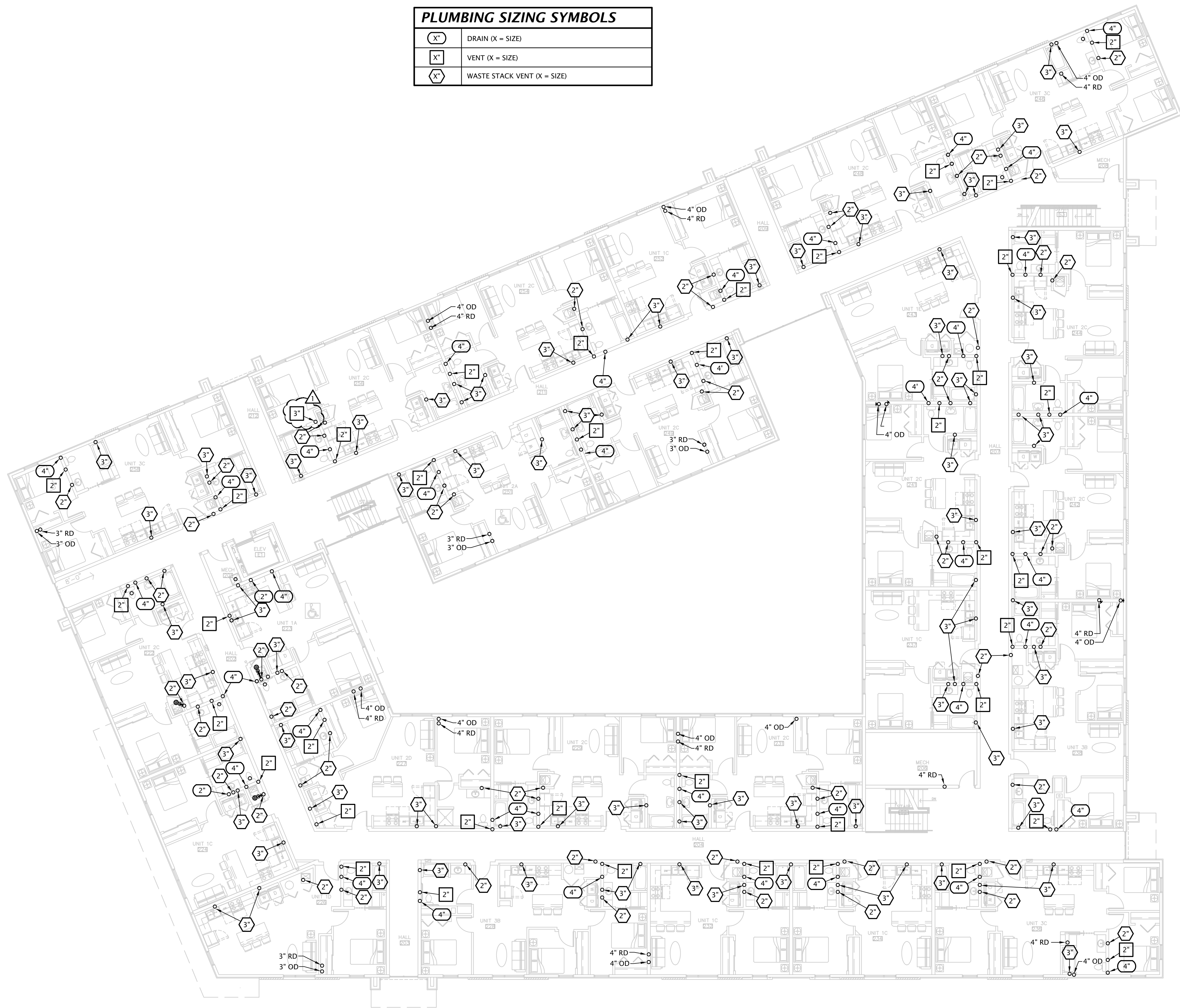
1 SECOND FLOOR PLAN - DRAIN AND VENT 3/32" = 1'-0"
