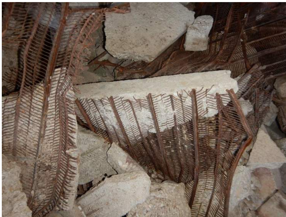
Photo 2: Detail of Berloy Ribplex from demo material pile
