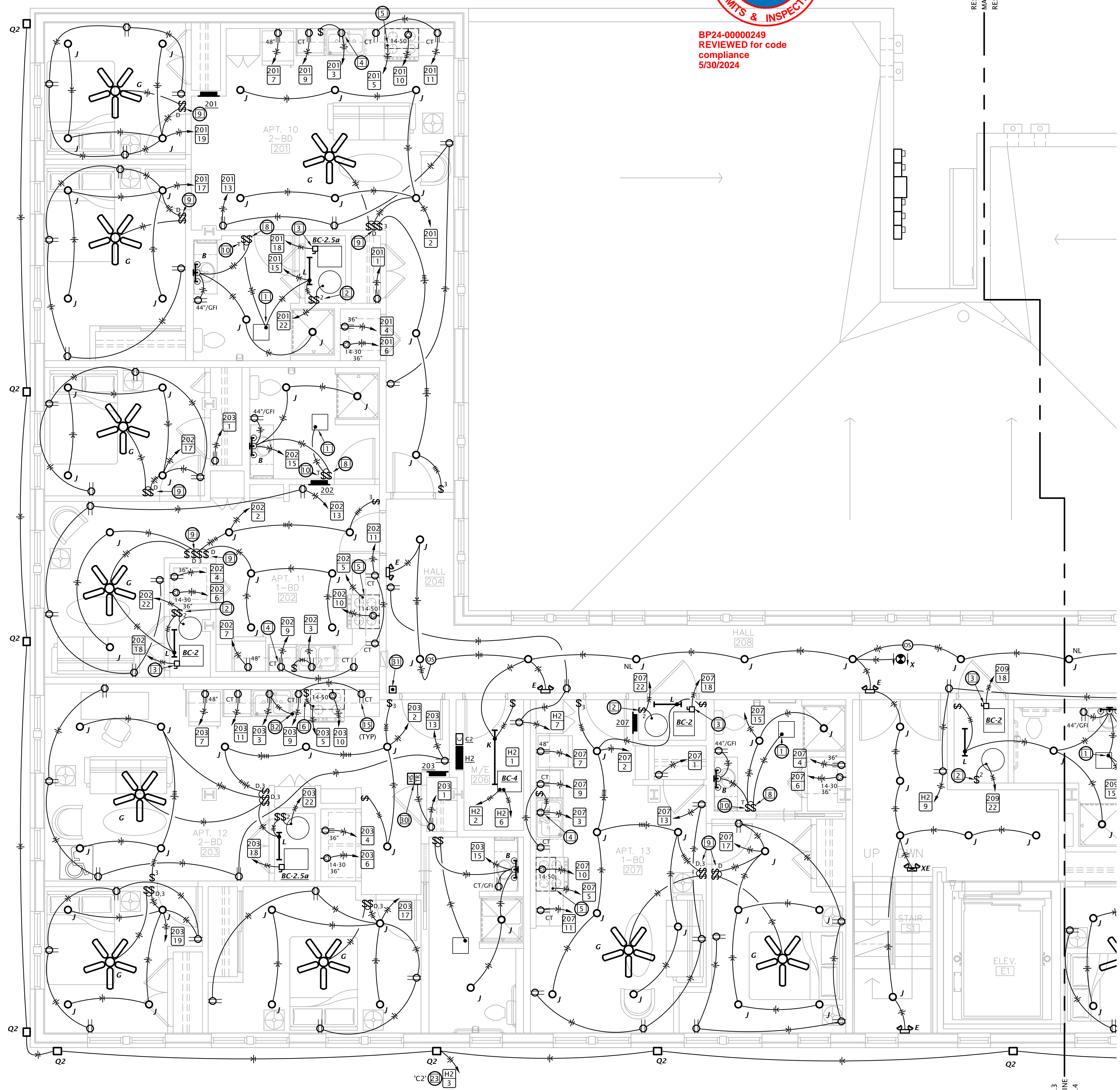
PARTIAL SECOND FLOOR ELECTRICAL PLAN 1/4" = 1'-0"
