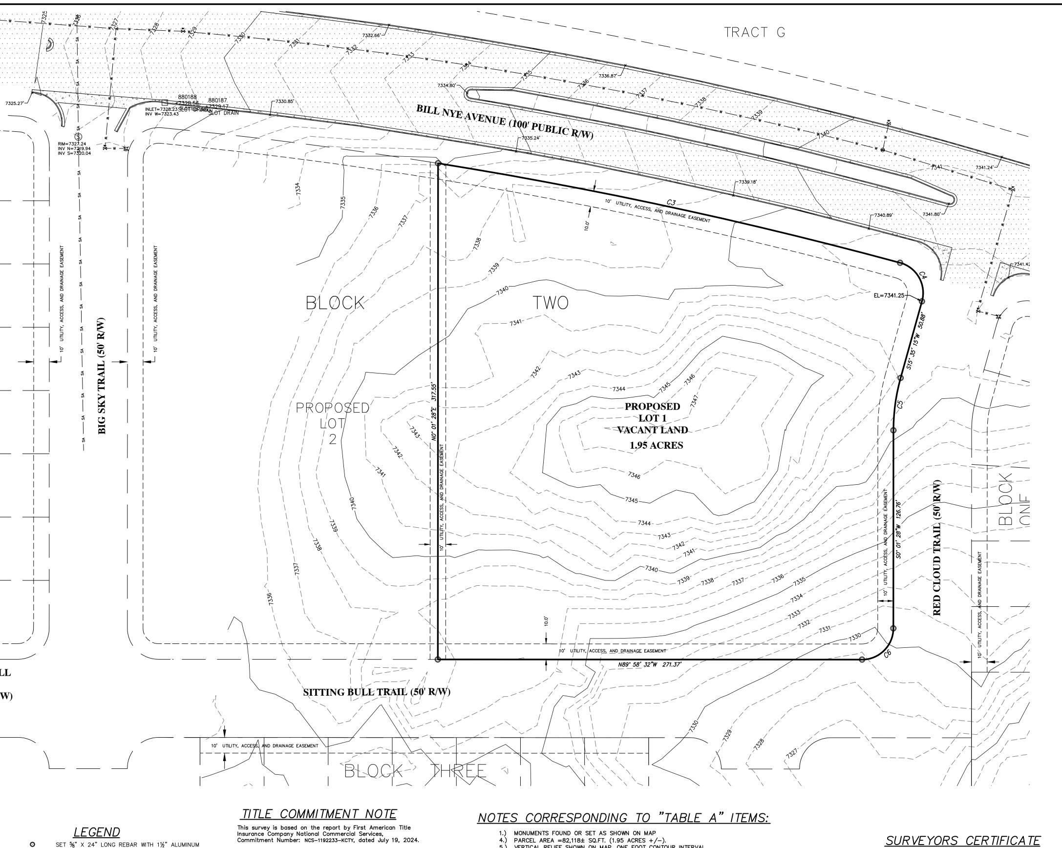
BASIS OF BEARINGS: WYOMING STATE PLANE COORDINATES, EAST ZONE, NAD83-2011, US SURVEY FEET, DISTANCES ARE GRID DISTANCES. ELEVATIONS: NAVD88
