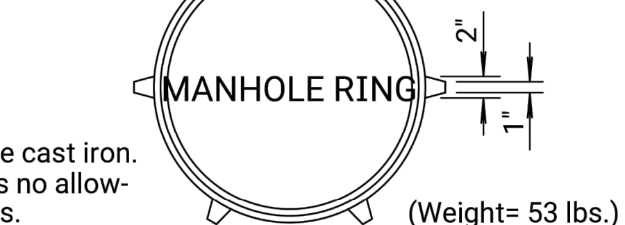
* LIGHT TYPE MANHOLE COVER & RING
