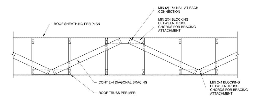
4 ROOF TRUSS BRACING 8521 3/4" = 1'-0"
