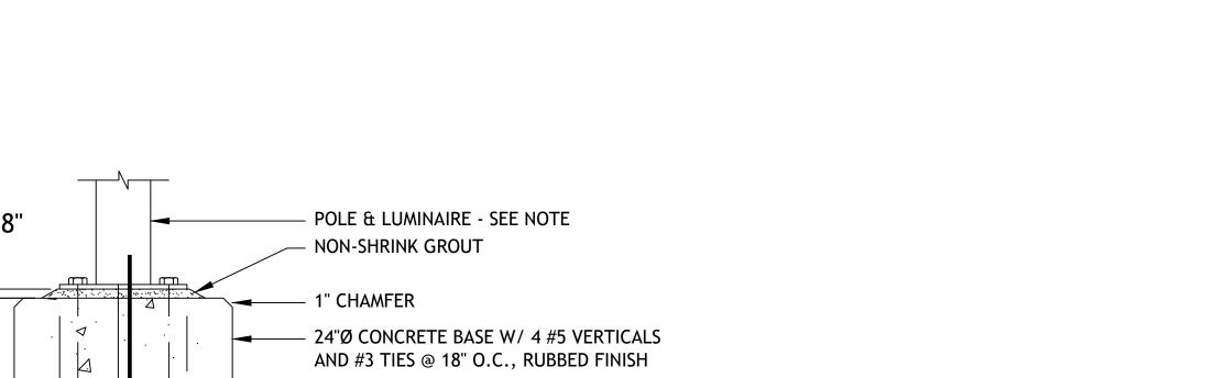
5/8" COPPERWELD GROUND ROD CONNECTED TO EQUIPMENT GROUNDWIRE AT GROUND LUG IN POLE ANCHOR BOLTS PER MFR'S REQUIREMENTS ELECTRICAL #4 BARS CONDUIT - 2" MIN. 3,000 PSI CONCRETE NOTE: 1. EXPANSION, CONTRACTION, OR CONSTRUCTION JOINTS ARE TO BE SAME AS NOTED ON TYPE "A" CURB AND GUTTER DETAIL. 2. REBAR IS NOT REQUIRED FOR CURB CONSTRUCTION ON A MINIMUM OF 3" ASPHALT. LUMINAIRE: SEE ARCH. PLANS
