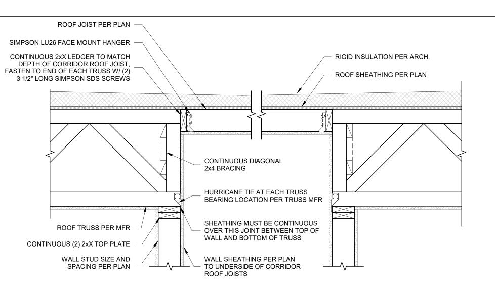
3 ROOF FRAMING SECTION AT CORRIDOR ROOF 5521 1" = 1'-0"
