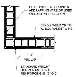
JOINT REINFORCING AT 3 \ INTERSECTING CMU WALLS  $\sqrt{5515}$  3/4" = 1'-0"
