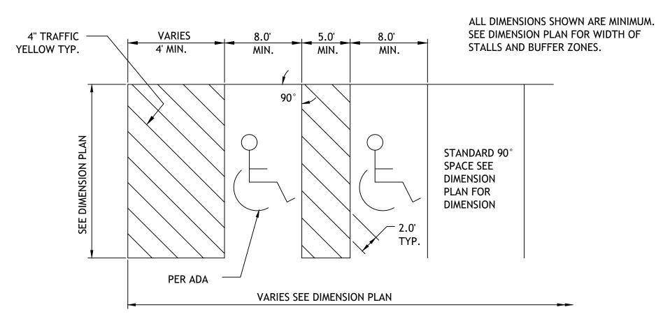
NOTE: PARKING SPACES AND ACCESS ISLES SHALL BE LEVEL WITH SURFACE SLOPES NOT EXCEEDING 1:50 IN ALL DIRECTIONS
