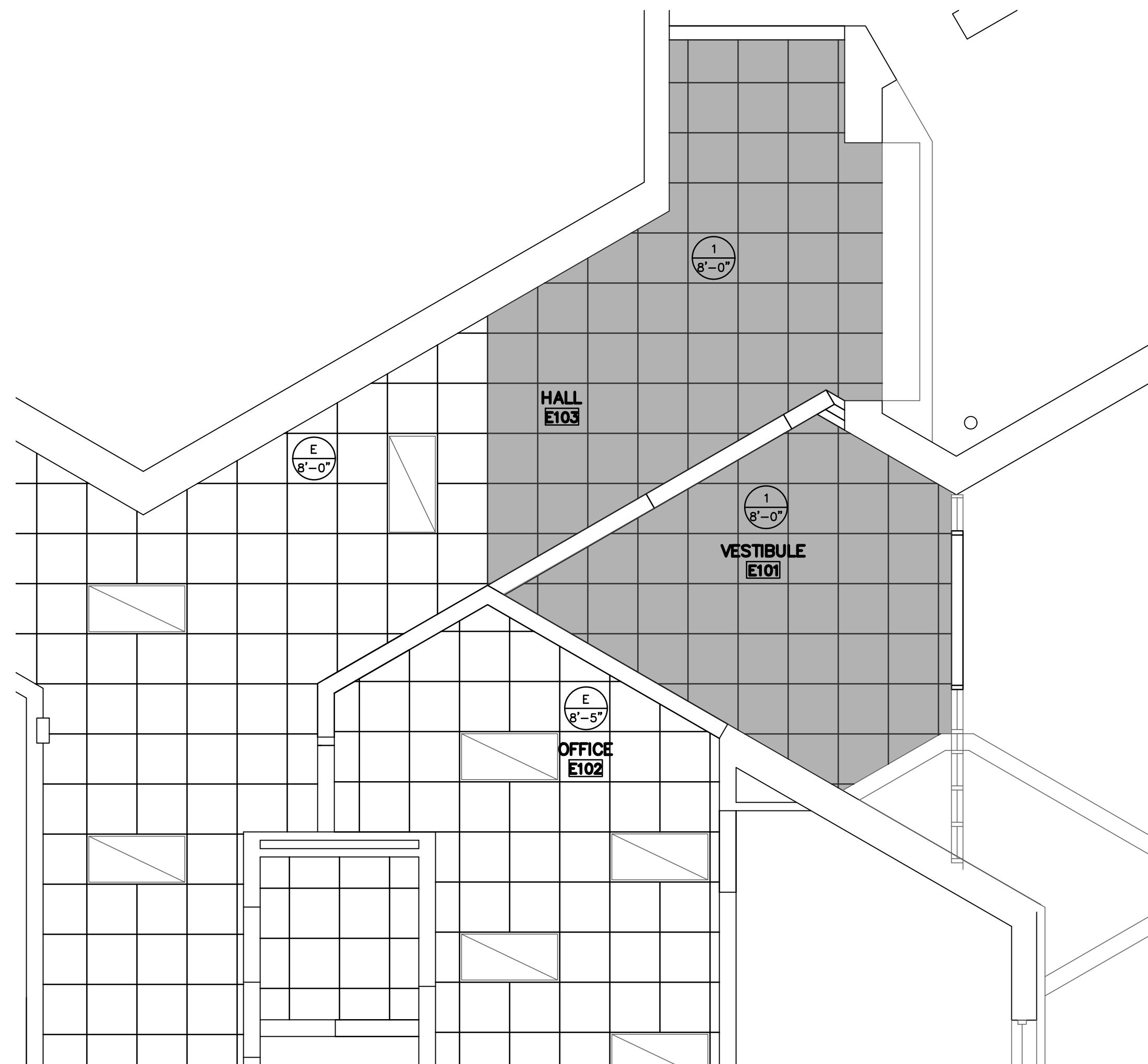
B ELEMENTARY SCHOOL FIRST FLOOR REFLECTED CEILING PLAN 1/4"=1'-0"
