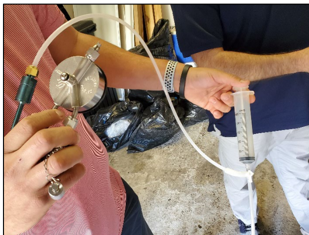
Image 7 – Set up leak-test assembly
