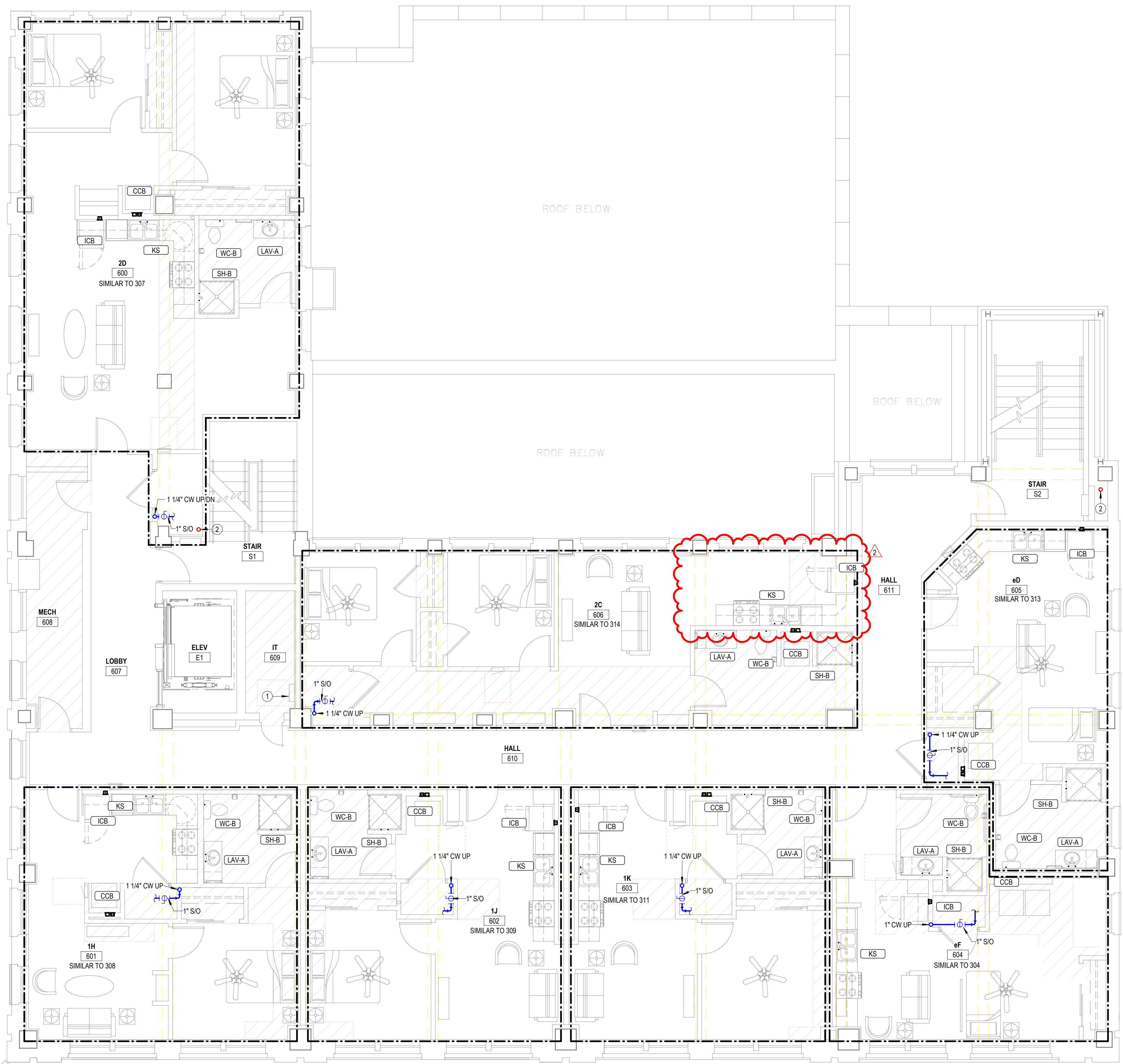
1 DOMESTIC WATER-SIXTH FLOOR PLAN 3/16" = 1'-0"
