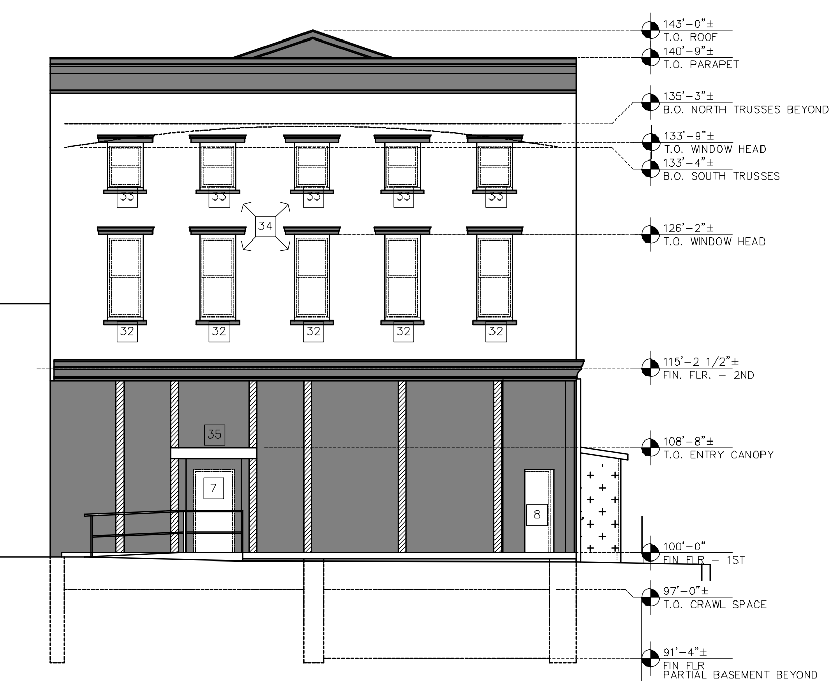
B DEMOLITION SOUTH/FRONT ELEVATION 1/8"=1'-0"
